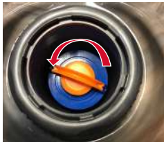
Turn Filters Counter-clockwise to Remove
