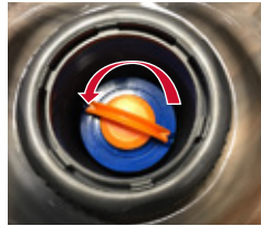
Turn Filters Counter-clockwise to Remove
