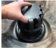
Pull Up to Remove Floater Assembly
