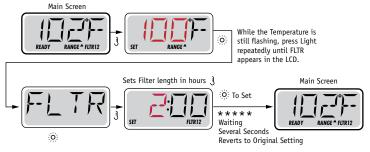
If Filter Cycle 2 is enabled, filtration indication of "12" will appear in the LCD. If filter cycle 2 is disabled, only filtration "1" will appear. This cannot be changed through the simple menu on this control panel and is based on the control system present (as to whether the system will do 1 cycle per day or 2 per day).
