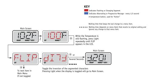
**NOTE:** Some panels may have a dedicated **FLIP** button, which allows the user to flip the display with a single button-press.
