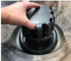
*Pull Up to Remove Floater Assembly*
