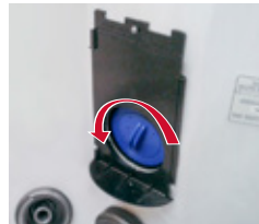
Turn Filters Counter-clockwise to Remove
