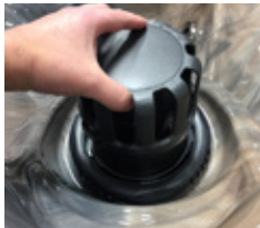
Pull Up to Remove Floater Assembly
