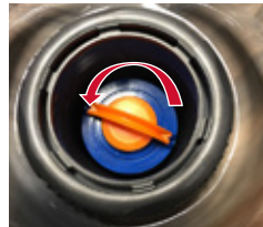
Turn Filters Counter-clockwise to Remove
