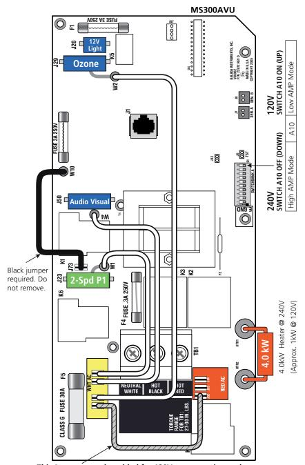
This Jumper must be added for 120V power option and DIP A10 must be ON. Remove Jumper for 240V hookup.
