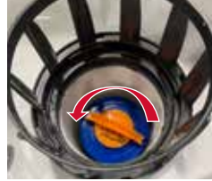
Turn Filters Counter-clockwise to Remove
