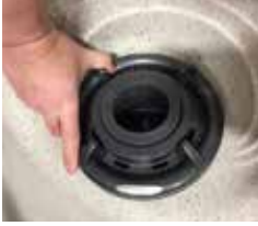
Twist Lock Ring Counter-clockwise to Remove Floater
