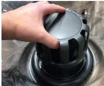
Pull Up to Remove Floater Assembly
