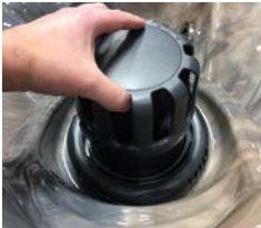
Pull Up to Remove Floater Assembly
