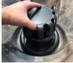
Pull Up to Remove Floater Assembly
