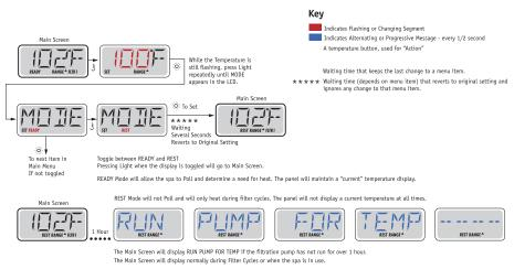
If the filtration pump has been off for an hour or more, when any function button, EXCEPT Light, is pressed on the panel, the pump used in conjuncton with the heater will run so that temperature can be sensed and displayed.
