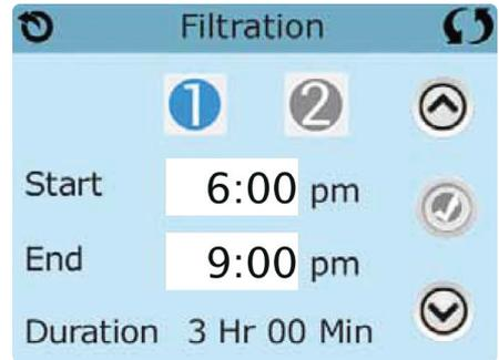
Press "1" to view Filter 1. Press "2" once to view Filter 2. Press "2" again to turn Filter 2 ON or OFF. When Filter Cycle 2 is ON, it can be adjusted in the same manner as Filter Cycle 1.
