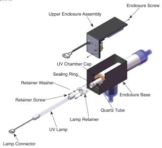
Figure 2: Spa Solar Eclipse Exploded View
