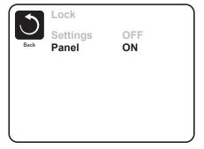
When the system is locked an icon will appear in the lower right hand corner of the display.
