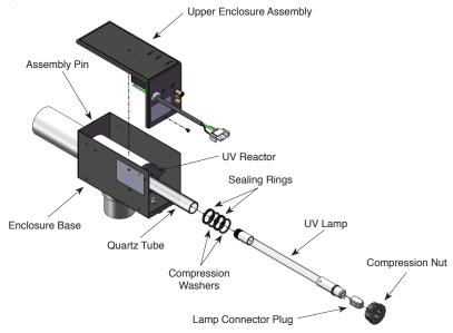
Figure 2: Mast3rPur System Exploded View
