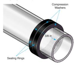
Figure 3: Quartz Tube Seal Assembly Detail
