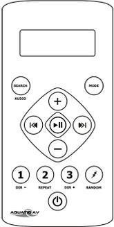
**i** In order to prolong remote battery life the LCD will shut off in 20 seconds if no other button is pressed. To turn remote back on press any key once and then press the command desired.
