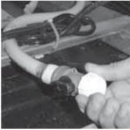
1. **DRAINING YOUR SPA.** The drain is located behind the front panel on the far right side, grasp the hose bib cap and turn it counter clockwise. Attach a garden hose, if desired. Turn the black knob on the side of the valve a quarter turn. Draining times may vary by model using the external hose bib. A sump pump may also be used to drain the spa quickly.
