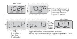
The control can be restricted to prevent unwanted use or temperature adjustments.
