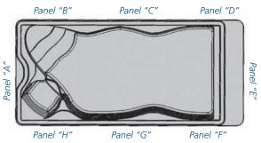
**NOTE:** The above drawing illustrates panel placement on the H2X. The CrossTrainer is labeled the same. **WARNING:** Do Not Remove Access Panels Without Turning Off Power To The Swim Spa.
