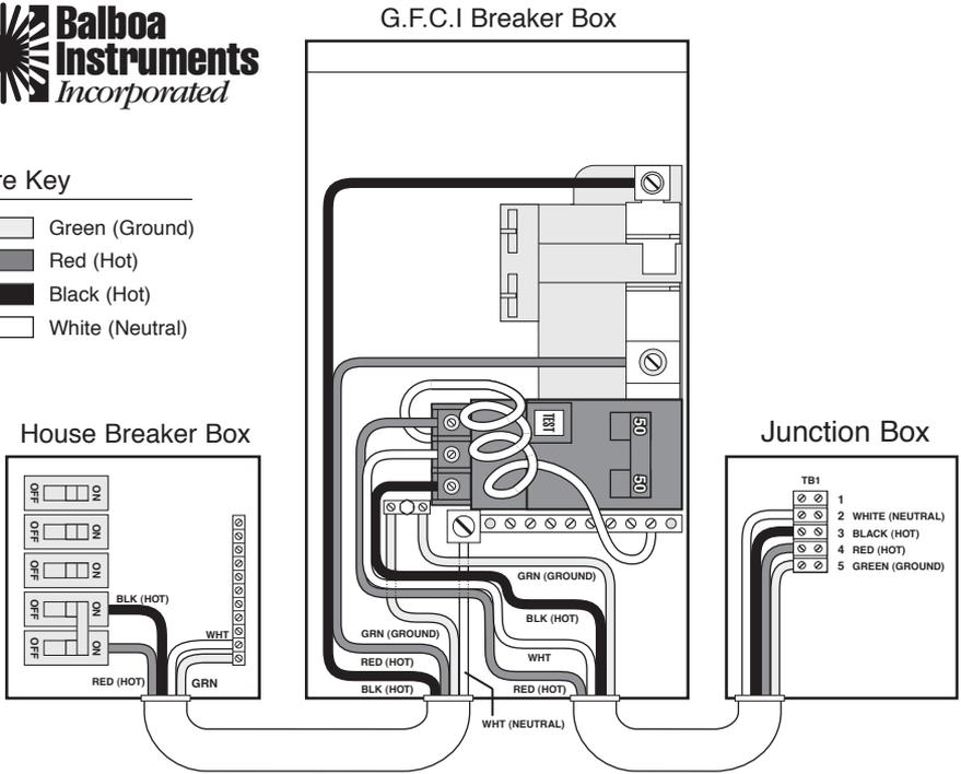
\* Actual wiring of GFCI will vary by manufacturer of GFCI. The GFCI shown is a Square D. Improper wiring of GFCI may result in permanent damage to spa system box. Repair / replacement of spa system box is not covered under warranty when damage results from improper wiring.
