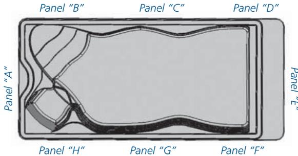
**NOTE:** The above drawing illustrates panel placement on the H2X. The CrossTrainer is labeled the same.
