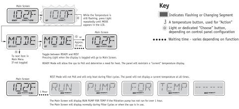
If the filtration pump has been off for an hour or more, when any function button, EXCEPT Light, is pressed on the panel, the pump used in conjuncton with the heater will run so that temperature can be sensed and displayed.
