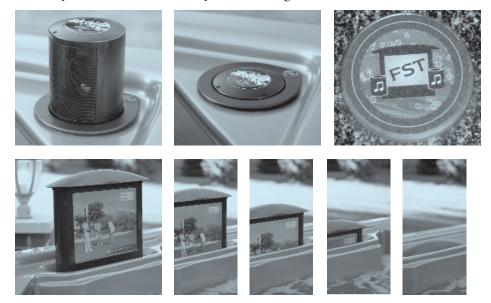
The TV and pop up speakers can be raised and lowered by pressing the one touch up and down FST auxillary button. Be sure the TV and speakers are down before placing the cover on the spa. Resulting damage is not covered under warranty if the cover is installed while the TV and speakers are still in the upright position.
