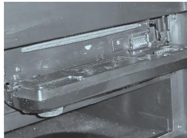
The Sony Stereo is shipped with the detachable stereo face in the spa's luggage pack. The stereo face must be inserted to operate any stereo functions.
