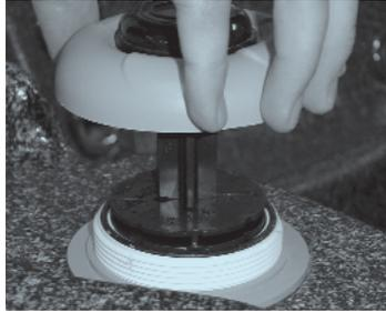
Turn the cap piece counter clockwise. It may be necessary to put a clean rag over the cap and turn it with a wrench.
