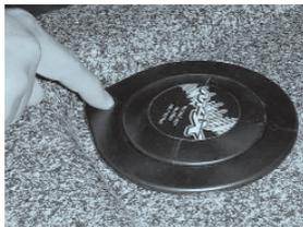
To use the pop-up speaker system, depress the button located in the corner. This will automatically raise the speaker for use.
